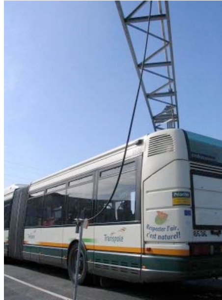
Bus filling station (mix natural gas/biomethane)
